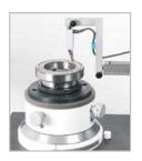
Precision measurement of Roundness, Cylindrical form and Straightness
